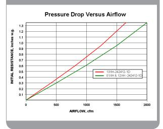
Camfil Farr high-capacity absolute filters are manufactured from the highest quality components, under demanding quality control conditions, and are certified to ensure performance in the most critical of applications. The XH is available in efficiencies from 99.97% to 99.999% on 0.3 micron particles. The XH is your choice for HEPA level air filtration in applications wherein ultra-clean air, increased airflow capacity and energy-savings are critical. Each Camfil Farr XH absolute includes:
